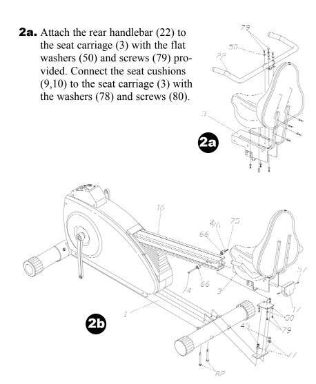
**2b.** First remove the support tube (24), from the main frame (1). Slide the assembled seat carriage onto the carriage tube (16). Re-assemble the support tube (24). Attach the end cap (17) with screws (57) and rear carriage tube rubber stopers (66) with bolts (74, 75) and washer (76).
